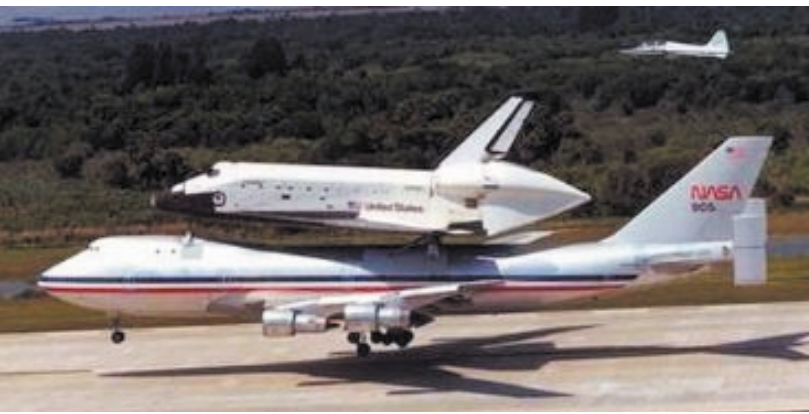
Figure 5.62 When the shuttle lands in California, it is returned to Florida on the back of a Boeing 747. The shuttle is almost as big as the commuter jets that fly from Edmonton to Calgary.
