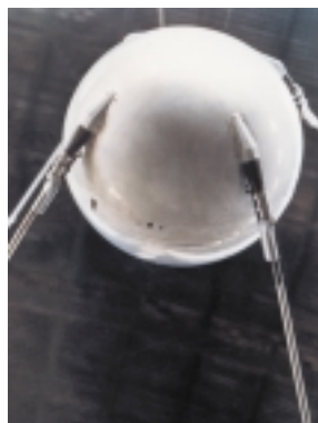
Figure 5.58 Sputnik 1 was the world's first artificial satellite. It was only about the size of a basketball and weighed 83 kg. It took about 98 min to orbit Earth. This was a great achievement and marked the beginning of the space age for humankind.
