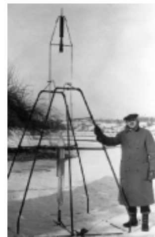
Figure 5.40 This is Dr. Robert Goddard and his first successful liquid fuel rocket, which he launched in 1926. The whole rocket was over 2 m tall and made of two sections connected by rods in which the gasoline and oxygen flowed.
