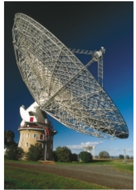
Figure 5.35 The collecting dishes of the first radio telescopes were huge compared to optical telescopes. Parke's radio telescope dish in New South Wales, Australia, is 64 m in diameter.
