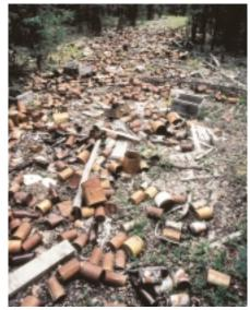
**Figure 2.60** The surface of a can that contains iron corrodes quickly outdoors. The rust formed on the surface of the can flakes off easily, so the can continues to corrode. The surface of an aluminum can oxidizes very quickly. The aluminum oxide formed makes a tough protective layer, which does not flake off easily. Therefore, aluminum cans will take over 400 years to degrade. How can you tell that most of the cans in this picture contain iron?
