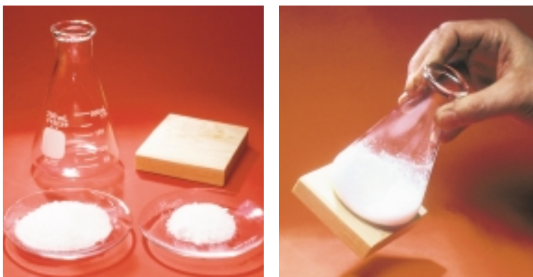
Figures 2.55 When ammonium thiocyanate and barium hydroxide octahydrate are mixed, an endothermic reaction occurs. Heat is absorbed from the surroundings. The Erlenmeyer flask becomes very cold. If water is placed on the bottom of the flask, it will freeze the flask to a wooden block.
