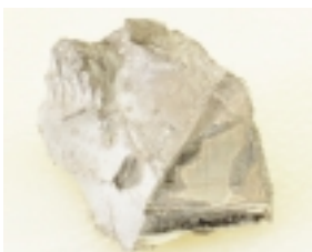
Figure 2.27B After a few minutes' exposure the surface of the sodium has dulled because the sodium atoms have reacted with oxygen from the air.
