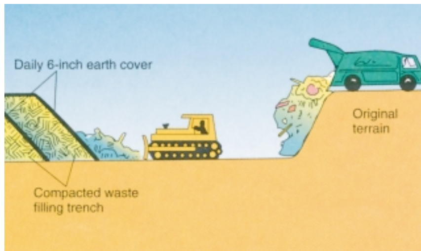
Figure 3.34 In a sanitary landfill, trash and garbage are crushed and covered each day to prevent accumulation of vermin and spread of disease. A waterproof lining is now required to prevent leaching of chemicals into ground water.
