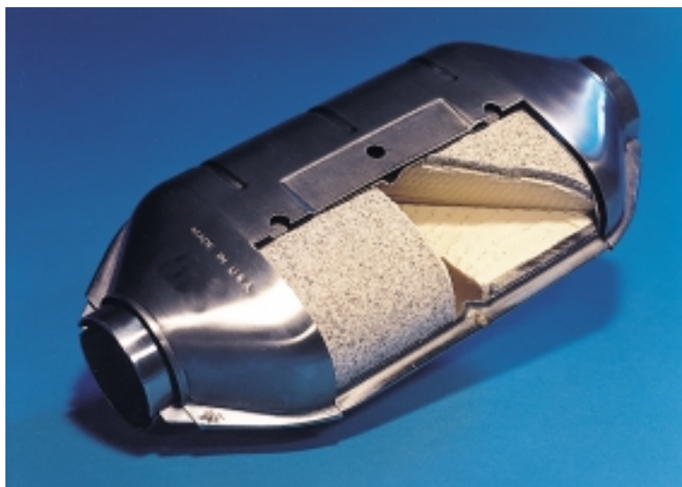
Figure 3.14 While catalytic converters are quite efficient, they work best when the catalysts are warmed up. It takes about 90 s, after a car starts, for the catalysts to be activated. Unfortunately, it is during this brief warm-up that the car produces about 70 percent of all the pollutants that it releases during its driving cycle.
