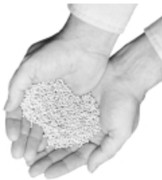
Figure 3.16 These little beads pack a big punch by removing sulfur dioxide and nitrogen oxides — pollutants responsible for acid precipitation — from gas given off during coal combustion.
