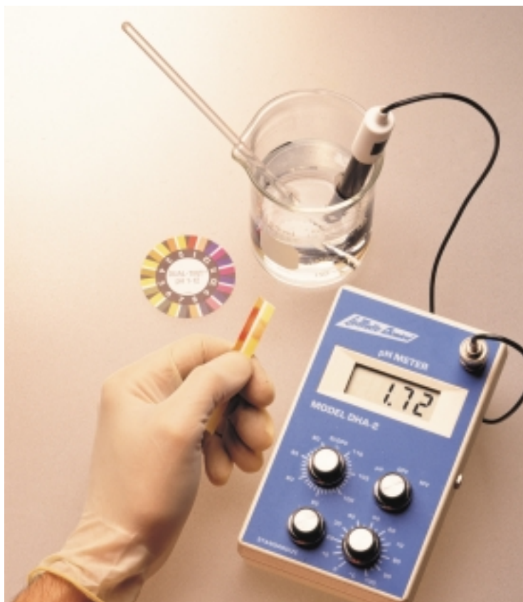
Figure 3.8 There are several ways to determine the pH of a substance. A pH meter and pH paper are two ways shown here.
