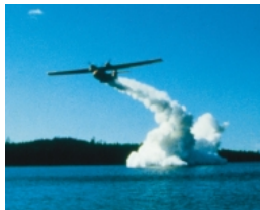
Figure 3.13 Liming is done by releasing powdered calcium carbonate from aircraft.
