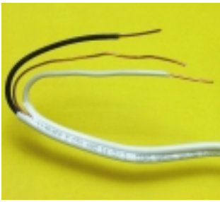
Figure 4.44 Fourteen gauge electric cable, commonly used for home wiring. Black = hot, white = neutral, bare copper (sometimes green) = ground.
