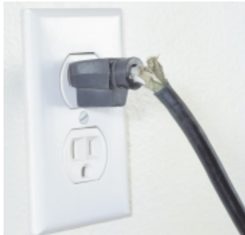
Figure 4.50 Frayed electrical cords are a serious shock and fire hazard.
