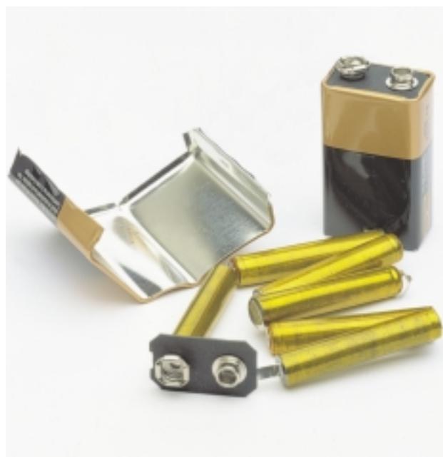
Figure 4.31 A 9 V battery contains six small 1.5 V cells. Are they connected in series or in parallel?
