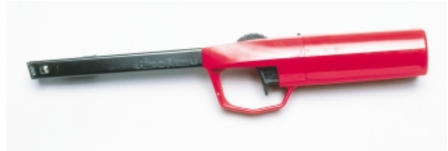
Figure 4.26 Squeezing the handle of a barbecue spark lighter slams a tiny hammer against a piezoelectric crystal, generating a potential difference of thousands of volts and a miniature lightning bolt across the spark gap.
