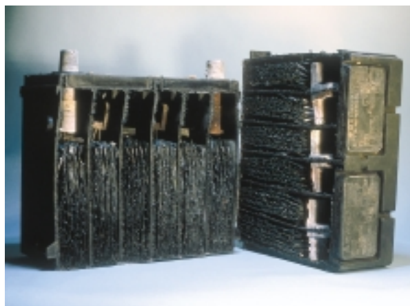
Figure 4.12 Chemical reactions inside the six cells of this car battery separate electrical charges, increasing their energy.
